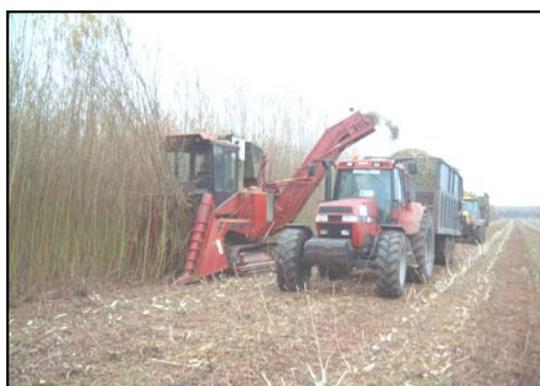
The harvesting method used by RES Ltd. is the billet harvesting system. This is harvesting with a self-propelled converted sugar cane harvester, with a converted head to cut the willow. The standard cutter box remains to leave the SRC fuel as billets. The harvester cuts the SRC into 150mm to 200mm lengths (billets) and discharges into trailers. Billets are typically 9mm (diameter) x 200mm (length) with the bark
