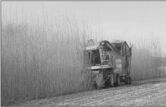
Short-rotation willow coppice is harvested every three to five years, during winter when the soil is frozen, using specially designed machines
